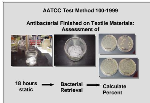
Fig. 3. AATCC Test Method 100-1999
