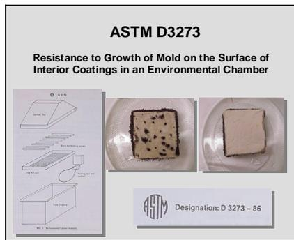
Fig. 5. ASTM Test Method D3273
