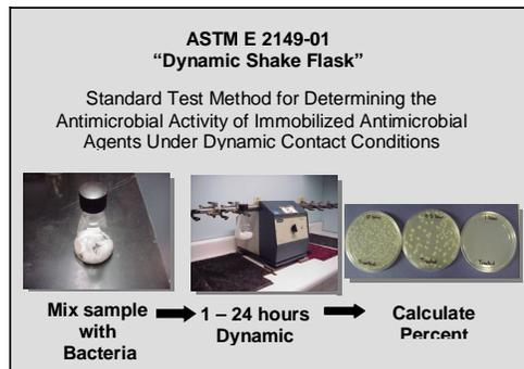
Fig. 2. Dynamic Shake Flask Test
